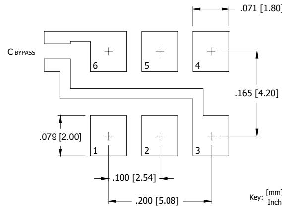
$C_{BYPASS}$  should be  $\geq 0.01 \mu\text{F}$ .
