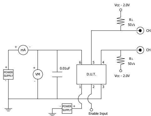
**TEST CIRCUIT, LVDS LOAD**
